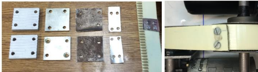
Figure 61 - Progression of Fastener Design and Final Fastened Lift Belt
